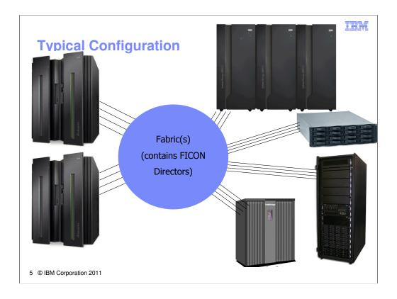
Shown here is a sample configuration. Processors and controllers are interconnected using one or more fabrics.
